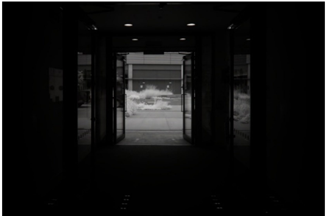
Fig. 2. Infrared photograph (~800–1000 nm) taken from inside the Here East building, showing infrared light only entering the building when the front doors are opened. The interior space appears otherwise completely dark as infrared light is not passed by the glazing.
